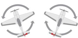
When the plane is rotated to left or right (Yaw), rudders should have the correcting actions as illustrated above.
