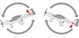
When the plane is rotated up or down (Pitch). elevators should have the correcting actions
