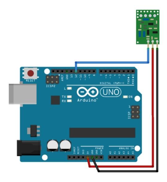
**Note**: always check the pinout for the transmitter module you're using. Usually, there are labels next to the pins. Alternatively, you can also take a look at your module's datasheet.
