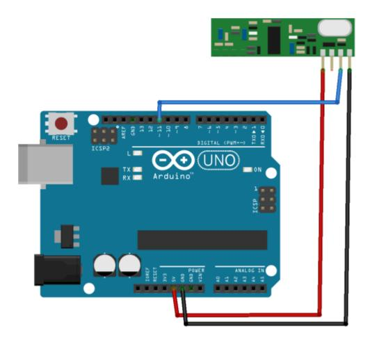
**Note**: always check the pinout for the receiver module you're using. Usually, there are labels next to the pins. Alternatively, you can also take a look at your module's datasheet.
