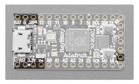
• The ItsyBitsy RP2040 has a Micro USB connector on the left in the image above. This connector is used to power and program the board. Use a Micro USB cable to plug the ItsyBitsy into your computer.
