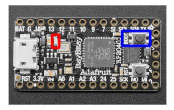
The little red LED (indicated by the red box) is located on the board near the 13 an 12 labels on the silk. The BOOT button (indicated by the blue
