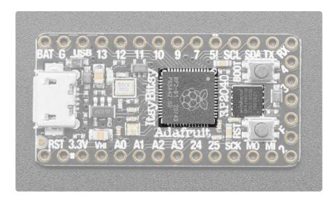
The square towards the middle is the RP2040 microcontroller, the "brains" of the ItsyBitsy RP2040 board.
