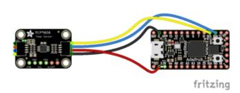
The black wire connects GND on the MCP9808 to ground on your board. The red wire connects VIN on the MCP9808 to power on your board. The yellow wire connects SCL on the MCP9808 to SCL on your board. The blue wire connects SDA on the MCP9808 to SDA on your board.
