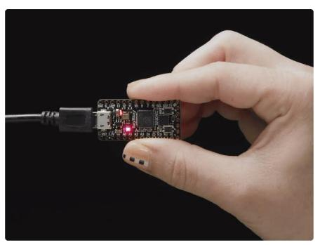
A new chip means a new ItsyBitsy, and the Raspberry Pi RP2040 is no exception. When we saw this chip we thought "this chip is going to be awesome when we give it the ItsyBitsy teensy-weensy treatment" and so we did! This Itsy' features the RP2040, and all niceties you know and love about the ItsyBitsy family (https://adafru.it/S4E)
