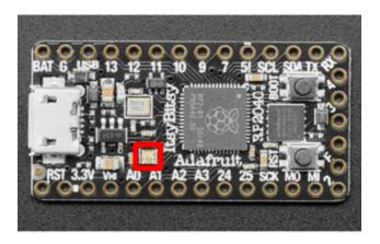
The NeoPixel LED (indicated by the red box in the image) is located near A0 and A1 on the board silk, next to the "Itsy" in "ItsyBitsy".
