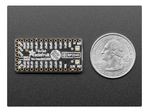
For peripherals, there are two I2C controllers, two SPI controllers, and two UARTs that are multiplexed across the GPIO - check the pinout for what pins can be set to which. There are 16 PWM channels, each pin has a channel it can be set to (ditto on the pinout).
