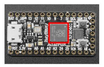
The CPU on your ItsyBitsy RP2040 is the big square located in the center of the board, inside of the "Adafruit ItsyBitsy RP2040" labels on the silk.
