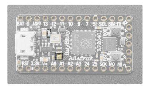
The little red LED is located towards the middle of the board between 13 and 12 on the silk. It is controllable in CircuitPython code using the pin **board.LED**. It is on RP2040 pin GPIO11.
