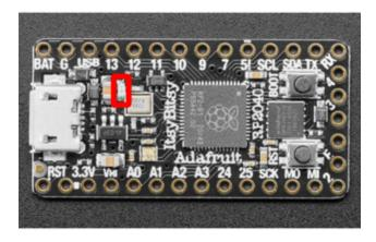
The little red LED (indicated by the red box) is located on the board near the 13 an 12 labels on the silk.
