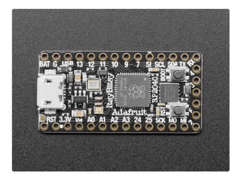
ItsyBitsy RP2040 is only 1.4" long by 0.7" wide, but has 6 power pins, 23 digital GPIO pins (4 of which can be analog in and 16 x PWM out). It's the same chip as the Feather RP2040 (http://adafru.it/4884) and Raspberry Pi Pico (http://adafru.it/4883) but really really small. So it's great once you've finished up a prototype, and want to make the project much smaller. It even comes with 8 MB of SPI Flash built in, for data logging, file storage, or CircuitPython/MicroPython code
