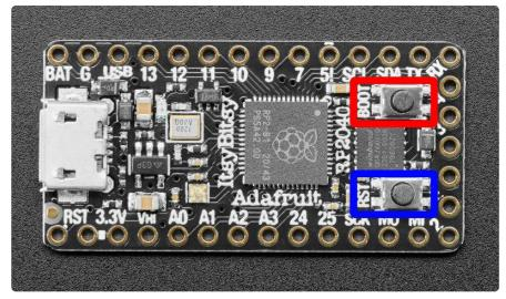
To enter the bootloader, hold down the BOOT/BOOTSEL button (highlighted in red above), and while continuing to hold it (don't let go!), press and release the reset button (highlighted in blue above). Continue to hold the BOOT/BOOTSEL button until the RPI-RP2 drive appears!
