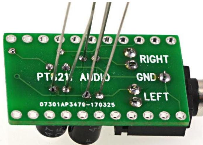
After all the parts are soldered, it's time to decide how your PT8211 board will connect with Teensy. In these photos, [ordinary pins](#) were soldered to the PT8211 board. You could choose to instead solder [sockets](#) to the PT8211, or use the [double insulator pins](#) to permanently join the two boards together.
