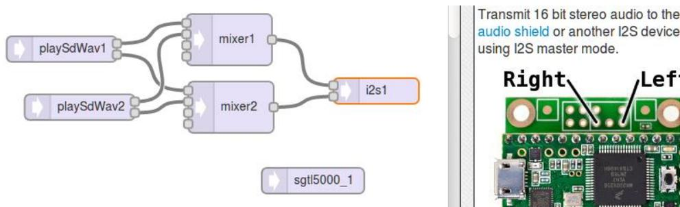
To convert this to PT8211, just delete the i2s1 output object and put a pt8211\_1 object in its place. Redraw the 2 connections. Also delete the sgtl5000\_1 object, since the PT8211 chip has no special control object.
