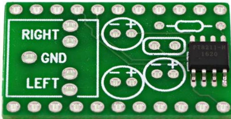
With the PT8211 tacked into place, carefully solder all 8 pins. This is the most
