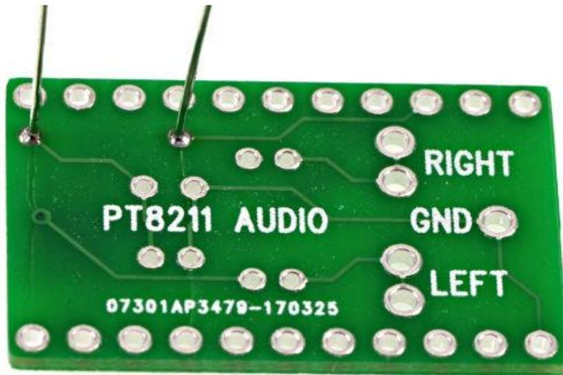
Then solder the 0.1  $\mu$ F capacitor. Like the resistor, this part is not directional.
